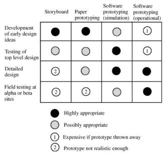
FIGURE 4. Application of different prototyping methods.
